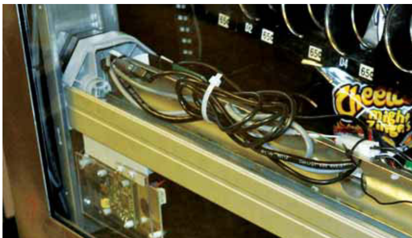
A digital camera rides on a track in the machine and takes pictures of individual products.
