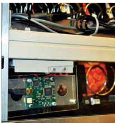
A digital camera rides on a track in the machine and takes pictures of individual products.
