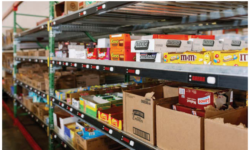
Legend Food Service’s snack lines are powered by Lightspeed Automation’s pick-to-light system to save time and improve “picking” accuracy.
