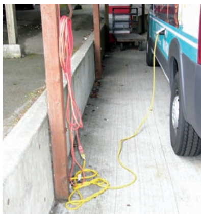
In the RAM ProMaster van, a 12-volt refrigerated compartment needs to be powered while the vehicle is off.
